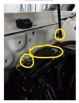
1. Fit and tighten ball stud to existing threaded hole as shown. You will have to reposition circled wiring loom, and anything else that may be in the way, like this earth wire perhaps, and the power outlet. The loom is quite ridgid, and I used adhesive foam to stop it vibrating
